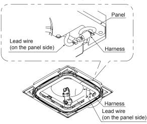
(3) Connect the connector of the lead wires and move the glass tube to cover the connector part.
