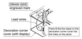
(3) Hook each of the cords of the remaining decoration corner covers (i.e., three covers) onto the corresponding pin on the panel.
