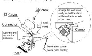
(2) Attach the decoration corner cover (with the display) to the corner with the <u>DRAIN SIDE</u> engraved mark. Push the connected lead wires through the corner hole onto the backside of the ceiling.
