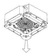
(1) Remove the bypass hole closing cap.
