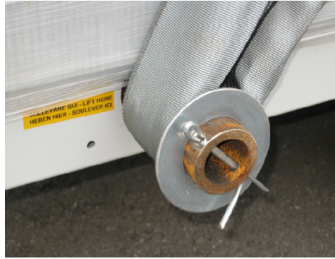
Fig. 3 Detail of hooking the sling to the lifting tube
